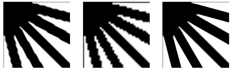
8 DDT using (a) Lawson's optimization, (b) bicubic reconstruction, and (c) DDT with look-ahead optimization.
